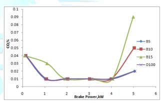
Fig -7: Variation of carbon monoxide with brake power
