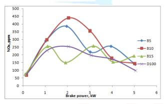
Fig 10 Variation of NOx with brake power
