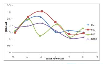
Fig 9 Variation of carbon dioxide with brake power
