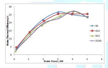
Fig 2 Variation of brake thermal efficiency with respect to brake power
